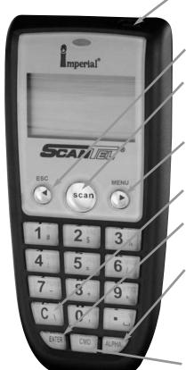
To power on the unit press the power key. The power key is on top right corner of the cover.
